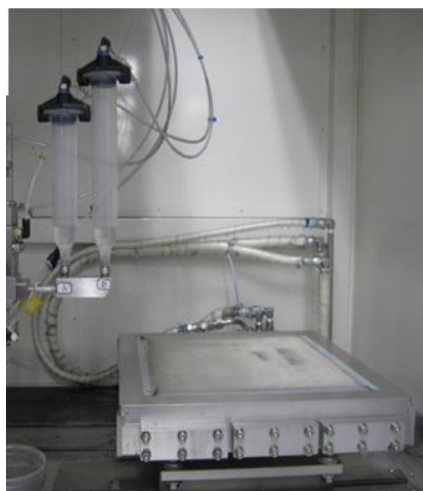
Fig. 3 Preparation of catalyst-coated membranes via pulse swirl spray method.
